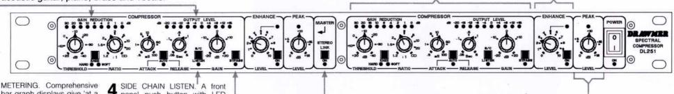
**3** METERING. Comprehensive bar graph displays give 'at a glance' indications of gain reduction, and input/output signal level. Gain reduction from -1dB to -30dB is shown simultaneously with signal level from -20dB to +15dB. Other single LEDs indicate function status of Hard/ Soft compression, Auto Attack/ Release, Side chain monitoring, Bypass, Enhancement, Peak Limiting, Stereo Linking and Power on.
