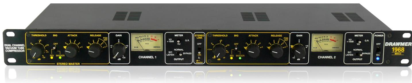
The 1968 MKII is a 1U Tube/FET 'stereo bus' compressor which by design delivers a transparent 'open' sound even during periods of heavy compression.
